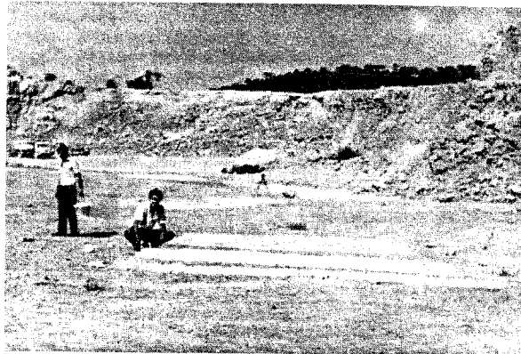
Photo 33.9. Field tests to measure the effectiveness of noise and air blast reduction in a detonating cord covered with sand.
