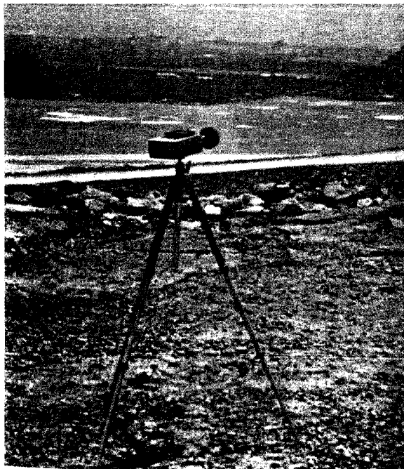
Photo 33.5. Sonometer installed to measure air blast.
