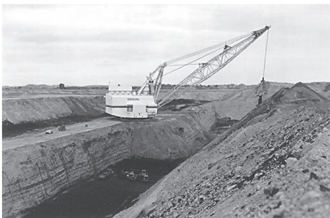
Figure 26.4 Overburden removal by a walking dragline.
