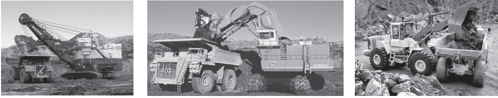
Figure 26.3 Loading of a dumper by using rope shovel, hydraulic shovel and front end loader.
