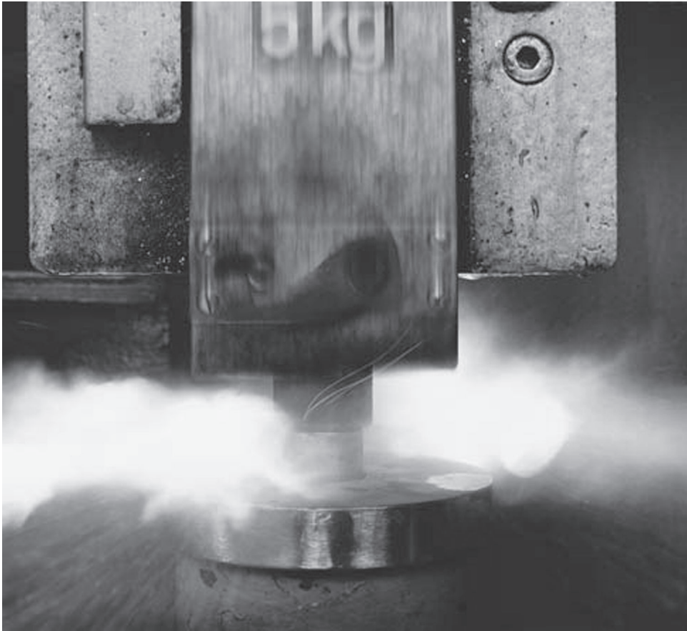
Figure 21.5 Drop weight test for measuring shock sensitivity.
