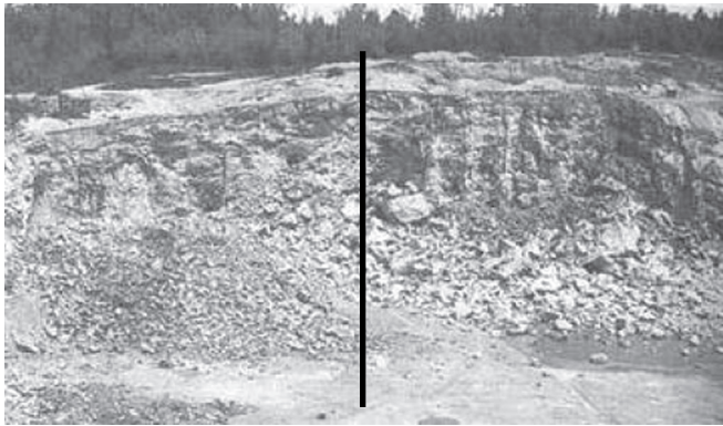
Figure 25.18 Difference between fragmentation achieved by delay based blast and instantaneous blast.
